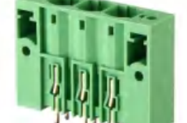
Pitch:10.16mm JL5EDGVM UL:300V/52A IEC:600V/57A Poles:2-8P
