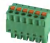
Pitch:3.5/3.81mm JL15EDGKD UL:300V/8A 28-16AWG IEC:250V/7A 1.5mm 2 Poles:2-24P
