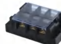
Pitch:12.00mm JL-250 UL:450V/30A 22-12AWG IEC:750V/32A 4.0mm 2 Poles:2-24P
