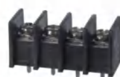
Pitch:9.50mm JL45C UL:300V/25A 22-12AWG IEC:750V/32A 2.5mm 2 Poles:2-24P
