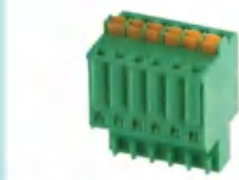
Pitch:2.50mm JL15EDGKD UL:125V/4A 28-20AWG IEC:250V/5A 0.5mm 2 Poles:2-24P
