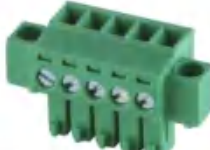
Pitch:3.5/3.81/5.08mm JL15EDGKM UL:300V/8A 28-16AWG IEC:250V/7A 1.5mm 2 Poles:2-24P
