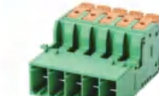
Pitch:7.62mm JL5EDGKHL UL:600V/37A 20-8AWG IEC:1000V/41A 6.0mm 2 Poles:2-12P
