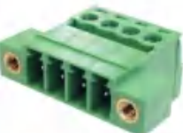
Pitch:3.5/3.81mm JL15EDGKRM UL:300V/8A 28-16AWG IEC:250V/7A 1.5mm 2 Poles:2-24P
