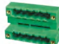
Pitch:5.00/5.08mm JL2EDGRMT UL:300V/15A IEC:320V/10A Poles:4-48P
