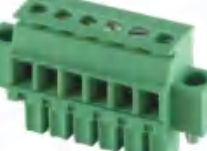
Pitch:3.5/3.81mm JL15EDGKBM UL:300V/8A 28-16AWG IEC:250V/7A 1.5mm 2 Poles:2-24P
