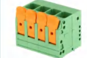
Pitch:10.0mm 可提供带错位针脚的型号 JL245V UL:600V/66A(1P) 300V/66A(2-12P)18-4AWG IEC:1000V/76A(1P) 630V/76A(2-12P)6.0mm² Poles:1-24P
