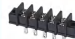
Pitch:8.25mm JL30H UL:300V/20A 22-14AWG IEC:300V/32A 2.5mm 2 Poles:2-24P
