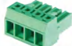
Pitch:7.62mm JL5EDGK UL:300V/30A 30-10AWG IEC:400V/32A 4.0mm 2 Poles:2-12P
