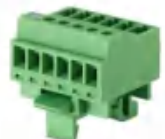
Pitch:3.81mm JL15EDG-VK UL:300V/8A 30-14AWG IEC:250V/7A 1.5mm² Poles:3-16P
