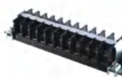
Pitch:11.5mm JLR30 UL:600V/35A 18-8AWG IEC:/ Poles:2-24P
