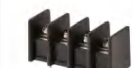
Pitch:9.5mm JL45C UL:300V/25A 22-12AWG IEC:750V/32A 2.5mm 2 Poles:2-24P
