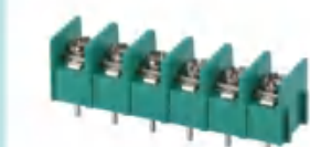
Pitch:7.62mm JL762B UL:300V/20A 22-14AWG IEC:250V/24A 2.5mm 2 Poles:2-24P
