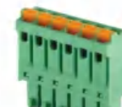
Pitch:3.50/3.81mm JL15EDGKN UL:300V/8A 28-16AWG IEC:250V/8A 1.0mm 2 Poles:2-24P
