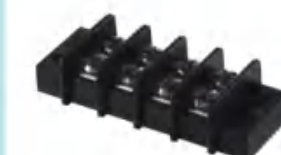
Pitch:9.50mm JL14 UL:300V/20A 22-12AWG IEC:450V/32A 4.0mm 2 Poles:2-24P
