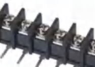
Pitch:8.25mm JL30R UL:300V/20A 22-14AWG IEC:450V/24A 2.5mm 2 Poles:2-24P
