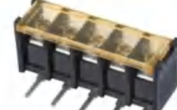
Pitch:9.50mm JL45RM UL:300V/25A 22-12AWG IEC:750V/32A 2.5mm 2 Poles:2-24P
