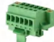
Pitch:3.81mm JL15EDG-VKM UL:300V/8A 30-14AWG IEC:250V/7A 1.5mm² Poles:3-16P
