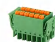
Pitch:3.50/3.81mm JL15EDGKNHCG UL:300V/8A 24-16AWG IEC:320V/8A 1.0mm² Poles:4-48P
