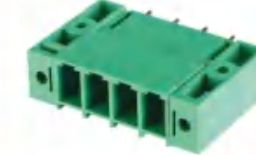
Pitch:7.62mm JL5EDGVM UL:300V/30A IEC:400V/32A Poles:2-12P
