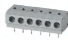
Pitch:3.81/3.96/5.00/7.50/10.00mm JL235W UL:300V/5A 20-18AWG IEC:250V/10A 1.5mm² Poles:2-24P
