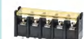
Pitch:8.25mm JL30CM UL:300V/20A 22-14AWG IEC:450V/24A 2.5mm 2 Poles:2-24P
