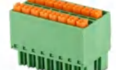
Pitch:3.50/3.81mm JL15EDGKNHC UL:300V/8A 24-16AWG IEC:320V/8A 1.0mm² Poles:4-48P
