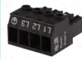
Pitch:7.62mm JL5EDGKH UL:600V/41A 24-8AWG IEC:1000V/41A 6.0mm 2 Poles:2-12P
