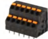
Pitch:5.0mm JL235H UL:300V/10A 28-16AWG IEC:630V/17.5A 1.5mm² Poles:4-48P
