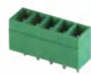
Pitch:3.5/3.81/5.08mm JL15EDGVC UL:300V/8A IEC:250V/7A Poles:2-24P
