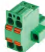
Pitch:5.00/5.08mm JL2EDGKDHM UL:300V/12A 26-12AWG IEC:320V/20A 2.5mm 2 Poles:2-24P
