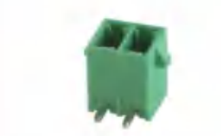
Pitch:3.50/3.81mm JL15EDGRN UL:300V/8A IEC:250V/7A Poles:2-24P
