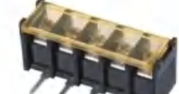
Pitch:8.25mm JL30RM UL:300V/20A 22-14AWG IEC:450V/24A 2.5mm 2 Poles:2-24P
