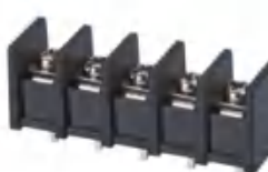
Pitch:10.00mm JL55S UL:300V/25A 22-12AWG IEC:750V/32A 4.0mm 2 Poles:2-24P
