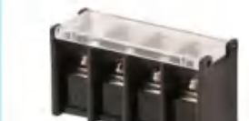
Pitch:9.5mm JL45CM UL:300V/25A 22-12AWG IEC:750V/32A 2.5mm 2 Poles:2-24P
