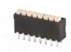
Pitch:3.5mm JL212V UL:300V/12A 28-14AWG IEC:320V/17.5A 1.5mm 2 Poles:2-24P
