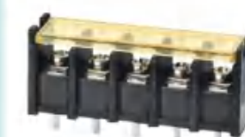
Pitch:11.00mm JL65CM UL:300V/25A 22-12AWG IEC:750V/32A 4.0mm 2 Poles:2-24P
