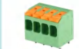
Pitch:7.5mm 可提供带错位针脚的型号 JL245R UL:600V/41A(1P) 300V/41A(2-12P) IEC:1000V/41A Poles:1-24P
