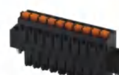
Pitch:3.50/3.81mm JL15EDGKNM UL:300V/8A 28-16AWG IEC:250V/7A 1.0mm 2 Poles:2-24P
