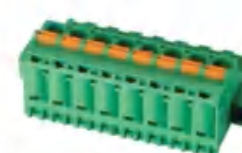
Pitch:5.0/5.08mm JL2EDGKDAM UL:300V/10A 24-14AWG IEC:320V/20A 2.5mm 2 Poles:2-24P
