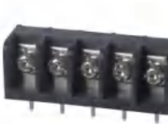
Pitch:9.50mm JL950(侧直针) UL:300V/25A 22-12AWG IEC:750V/32A 2.5mm 2 Poles:2-24P
