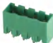
Pitch:5.00/5.08/7.60/7.62mm JL2EDGVC UL:300V/15A IEC:320V/20A Poles:2-24P
