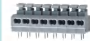
Pitch:3.81/3.96/5.00/7.50/10.00mm JL235T UL:300V/5A 20-18AWG IEC:750V/15A 1.5mm² Poles:2-24P
