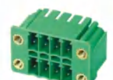
Pitch:3.50/3.81mm JL15EDGKNVM UL:300V/8A IEC:250V/7A Poles:4-48P
