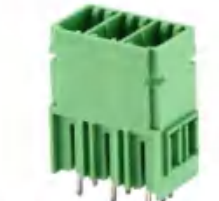
Pitch:7.62mm JL5EDGVHC UL:300V/41A IEC:1000V/41A Poles:2-12P
