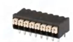
Pitch:3.5mm JL212R UL:300V/12A 28-14AWG IEC:320V/17.5A 1.5mm 2 Poles:2-24P
