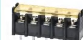
Pitch:8.50mm JL35CM UL:300V/20A 22-14AWG IEC:450V/32A 2.5mm 2 Poles:2-24P
