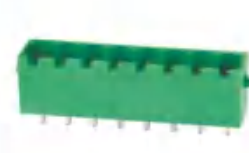
Pitch:5.00/5.08/7.50/7.62mm JL2EDGVN UL:300V/15A IEC:400V/20A Poles:2-24P
