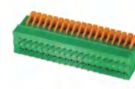
Pitch:2.54mm JL141V UL:150V/5A 26-20AWG IEC:130V/6A 1.0mm 2 Poles:1-24P
