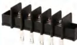
Pitch:9.5mm JL45H UL:300V/25A 22-12AWG IEC:750V/32A 2.5mm 2 Poles:2-24P
