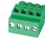
Pitch:5.00/5.08/7.62mm JL2EDGKB UL:300V/15A 28-12AWG IEC:320V/18A 2.5mm 2 Poles:2-24P
