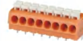
Pitch:5.00mm JL270 UL:300V/12A 28-12AWG IEC:250V/16A 0.2-2.5mm² Poles:2-24P
