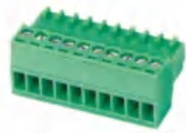
Pitch:2.54mm JL15EDGY UL:125V/4A 28-20AWG IEC:250V/5A 0.5mm 2 Poles:2-24P
