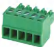
Pitch:3.5/3.81/5.08mm JL15EDGK UL:300V/8A 28-16AWG IEC:250V/7A 1.5mm 2 Poles:2-24P
