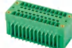
Pitch:3.50/3.81mm JL15EDGRHM UL:300V/8A IEC:320V/5A Poles:4-48P
