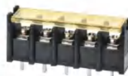
Pitch:10.00mm JL55CM UL:300V/25A 22-12AWG IEC:750V/32A 4.0mm 2 Poles:2-24P
