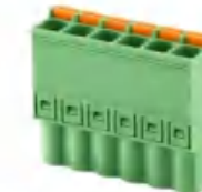
Pitch:5.08mm JL2EDGKN UL:300V/10A 24-12AWG IEC:320V/15A 2.5mm 2 Poles:2-24P
