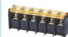
Pitch:10.00mm JL55SM UL:300V/25A 22-12AWG IEC:750V/32A 4.0mm 2 Poles:2-24P
