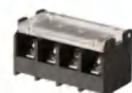
Pitch:7.62mm JL762M UL:300V/20A 22-14AWG IEC:250V/24A 2.5mm 2 Poles:2-24P
