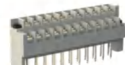
Pitch:7.62mm JL762D-7.62 UL:300V/10A 22-14AWG IEC:320V/15A 2.5mm 2 Poles:4-48P
