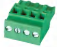
Pitch:5.00/5.08/7.62mm JL2EDGKA UL:300V/15A 28-12AWG IEC:320V/18A 2.5mm 2 Poles:2-24P
