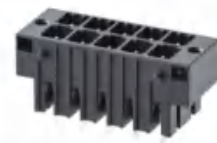
Pitch:5.08mm JL2EDGVHCM UL:300V/10A IEC:630V/8A Poles:4-48P
