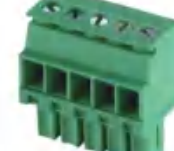
Pitch:3.5/3.81mm JL15EDGKB UL:300V/8A 28-16AWG IEC:250V/7A 1.5mm 2 Poles:2-24P
