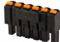
Pitch:7.62mm JL9EDGKD UL:600V/20A 20-12AWG IEC:1000V/20A 2.5mm 2 Poles:2-12P
