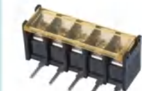
Pitch:11.00mm JL65RM UL:300V/25A 22-12AWG IEC:750V/32A 4.0mm 2 Poles:2-24P
