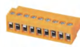
Pitch:3.96mm JL396 UL:300V/10A 26-14AWG IEC:160V/10A 1.5mm² Poles:2-24P
