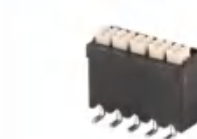
Pitch:3.5mm JL212V-SMT UL:300V/12A 28-14AWG IEC:320V/17.5A 1.5mm 2 Poles:2-24P
