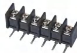
Pitch:9.50mm JL45R UL:300V/25A 22-12AWG IEC:750V/32A 2.5mm 2 Poles:2-24P
