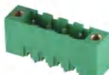
Pitch:5.00/5.08/7.60/7.62mm JL2EDGVM UL:300V/15A IEC:320V/20A Poles:2-24P
