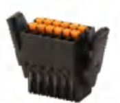
Pitch:2.54mm JL15EDGKDHL UL:150V/5A 30-20AWG IEC:320V/6A 0.5mm 2 Poles:4-48P
