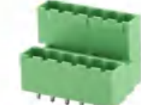
Pitch:5.08mm JL2EDGVTC UL:300V/15A IEC:320V/10A Poles:4-48P
