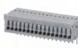
Pitch:2.54mm JL143R UL:150V/5A 24-20AWG IEC:130V/6A 1.0mm 2 Poles:2-24P
