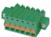
Pitch:3.5/3.81mm JL15EDGKDM UL:300V/8A 28-16AWG IEC:250V/7A 1.5mm 2 Poles:2-24P
