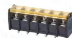
Pitch:8.25mm JL30SM UL:300V/20A 22-14AWG IEC:450V/24A 2.5mm 2 Poles:2-24P
