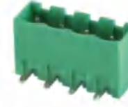
Pitch:5.00/5.08/7.60/7.62mm JL2EDGRC UL:300V/15A IEC:320V/20A Poles:2-24P
