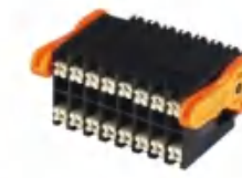
Pitch:3.50mm JL15EDGKNHBG UL:300V/10A 28-16AWG IEC:320V/13.4A 0.5-1.5mm² Poles:4-48P
