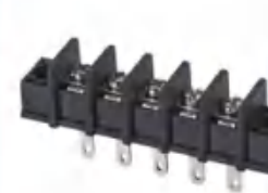
Pitch:11.00mm JL65H UL:300V/25A 22-12AWG IEC:750V/32A 4.0mm 2 Poles:2-24P
