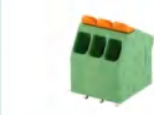
Pitch:7.5mm 可提供带错位针脚的型号 JL245S UL:600V/41A(1P) 300V/41A(2-12P) 24-8WG IEC:1000V/41A 6mm² Poles:1-24P
