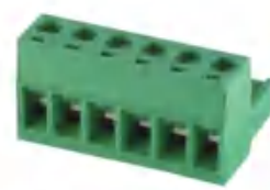
Pitch:5.08mm JL2EDGK-1000A UL:300V/20A 28-12AWG IEC:320V/15A 2.5mm 2 Poles:2-24P
