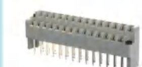
Pitch:7.62mm JL762A-7.62加高型 UL:300V/15A 22-14AWG IEC:320V/15A 2.5mm 2 Poles:4-48P
