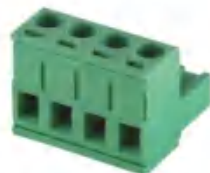
Pitch:5.00/5.08/7.60/7.62mm JL2EDGK UL:300V/15A 28-12AWG IEC:320V/20A 2.5mm 2 Poles:2-24P
