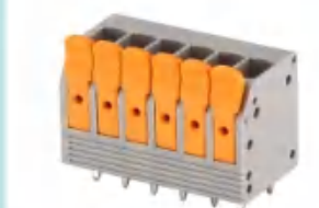
Pitch:5.0mm JL245V UL:300V/20A 24-12AWG IEC:630V/32A 4.0mm² Poles:1-24P
