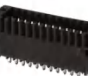
Pitch:2.54mm JL15EDGVHDM UL:150V/8A IEC:320V/10A Poles:4-48P
