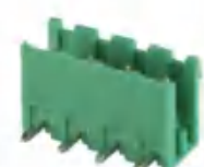
Pitch:5.00/5.08/7.60/7.62mm JL2EDGR UL:300V/15A IEC:320V/20A Poles:2-24P
