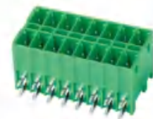
Pitch:3.50/3.81mm JL15EDGKNR UL:300V/8A IEC:250V/7A Poles:4-48P
