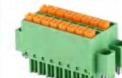
Pitch:3.50/3.81mm JL15EDGKNHCM UL:300V/8A 24-16AWG IEC:320V/8A Poles:4-48P
