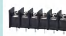
Pitch:11.00mm JL65C UL:300V/25A 22-12AWG IEC:750V/32A 4.0mm 2 Poles:2-24P
