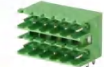
Pitch:5.08mm JL2EDGKRH UL:300V/10A IEC:630V/8A Poles:4-48P
