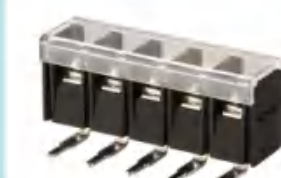
Pitch:9.5mm JL48R UL:300V/25A 22-12AWG IEC:750V/32A 2.5mm 2 Poles:2-24P
