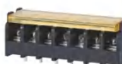
Pitch:8.25mm JL825M UL:300V/20A 22-14AWG IEC:500V/32A 2.5mm 2 Poles:2-24P
