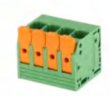
Pitch:7.5mm 可提供带错位针脚的型号 JL245V UL:600V/41A(1P) 300V/41A(2-12P)24-8AWG IEC:1000V/41A 6.0mm² Poles:1-24P
