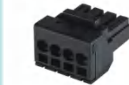
Pitch:5.0mm JL9EDGK UL:300V/14.5A 28-14AWG IEC:320V/20A 2.5mm 2 Poles:2-14P
